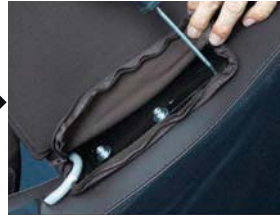
Tighten the screws Make sure holes are straight to screws
