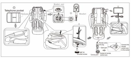
Put the back seat cushion, shoulder cushion, head pad onto the backrest and connect the two parts with zipper and velcro.
