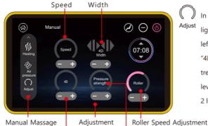
In the ON status, click the icon Adjust lights up, finger tough slide from left to right, to adjust the "speed" "4D width", time, 4D, pressure trength, roller speed. 4D has 4 level, width 3 level, roller speed 2 level. Click the " "," " + - to adjust.
