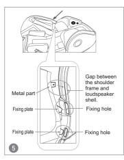
Insert the 2 metal fixingpart of the backarmrestinto the fixinghole on the backmain body, and insert the up fixingpart into the gap between shoulderframe and loudspeaker shell.
