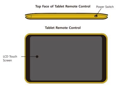
1. After the chair is powered on, the tablet will turn on by default and display the boot interface. After a while, enter the main interface and press the power switch at the right end of the top face of the tablet to turn on/off the display of the tablet.
